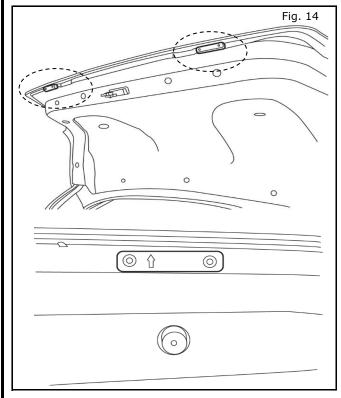
b) Install (2) rubber bumpers into open holes. Rubber bumpers must be installed with arrow pointing up and completely seated to trunk metal.
